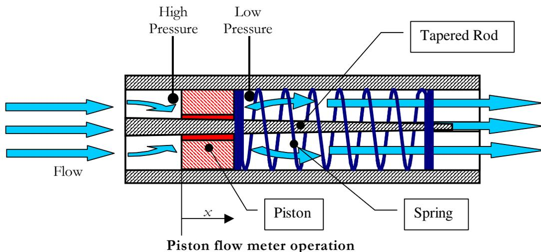
Typically, such flow meters provide an accuracy of about  $\pm 5\%$ . If this accuracy could be improved while maintaining cost competitiveness, a greater share of the expanding market would be captured. As a part of a project to improve the accuracy, the variability of the spring rate was considered. The instrumentation company asked that the quality of the springs be improved without an increase in cost.
